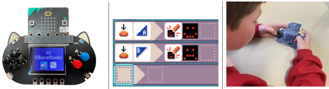
Fig. 1. The MicroCode physical computing system. On the left, micro:bit V2 inserted into a MicroCode shield and running MicroCode; in the centre, a screenshot of the MicroCode editor displaying the “Happy/Sad” program; at right, a student using MicroCode.
