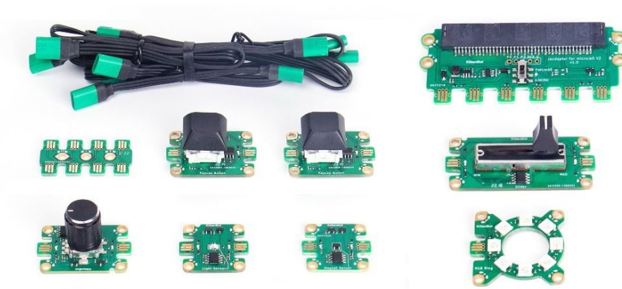
Figure 3: Jacdac modules created by KittenBot. From top left: Jacdac cables, Jacdac adapter for micro:bit, Jacdac hub, and seven Jacdac modules - two buttons, slider, rotary encoder, light and magnetic sensors, LED ring. Available at https://www.kittenbot.cc/collections/frontpage/products/kittenbot-jacdac-kit-for-micro-bit
