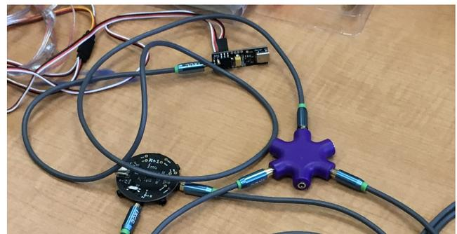
Figure 4: A Brain connected to a Motor Bead through a standard multi-way headphone splitter and audio cables.
